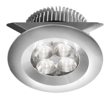
Aluminum 2x4W 3000K, CRI80+, 25° beam, 24VDC input with Male Connector, 18" Lead wire, D70xH50 mm, Dimmable.
