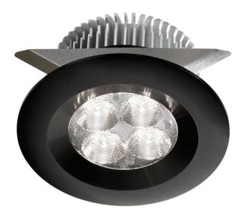
Black 2x4W 3000K, CRI80+, 25° beam, 24VDC input with Male Connector, 18" Lead wire, D70xH50 mm, Dimmable.
